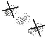
First put the bold and the plain washer through the slot of the smaller curved plate. Then, screw the nut flush onto the bolt, as shown in the picture at the right.
