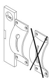
You may then connect the plates by putting the nut of the shorter plate through the slot on the longer plate. Then tighten the nut with the wrench to complete the installation.
